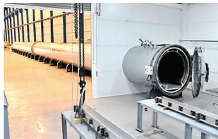
**An advanced CAD system operating throughout Persico and linked with rig-partners Future Fibres in Valencia allows only approved staff into the design and engineering process. Substantial milled aluminium spar mould (left) and dedicated autoclave (right)**
