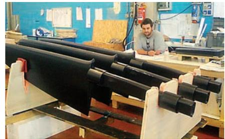
**Once the female tooling (left) is completed, making perfect rudders for a new VO70 becomes a ‘relatively’ straightforward process – and you don’t want to be running short**
