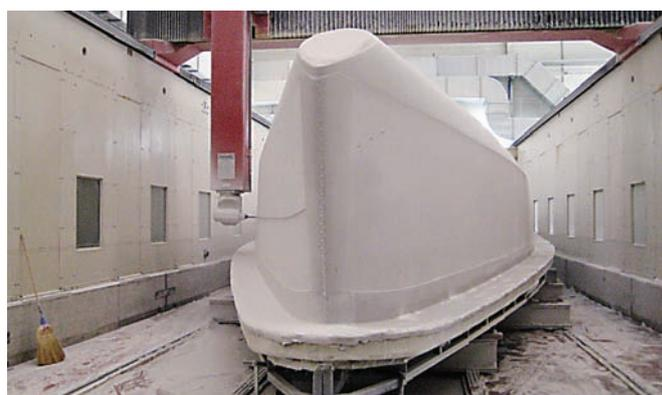
**Top:** Persico Marine built the hulls and many of the other major components for Italy's Luna Rossa's reliable and stiff AC72. **Above:** final CNC machining in Persico's expansive facility of the plug for the female hull moulds for the new Volvo VO65 fleet
