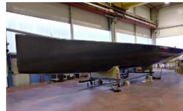
from strength to strength in a relatively short time. Typically we run with several teams on the shop floor, a hull shell team, a deck shell team and a components team. Once the deck is fitted a further team take care of all the vital secondary bonding and fit-out phase. This approach ensures extremely high quality while respecting the always challenging schedule.
